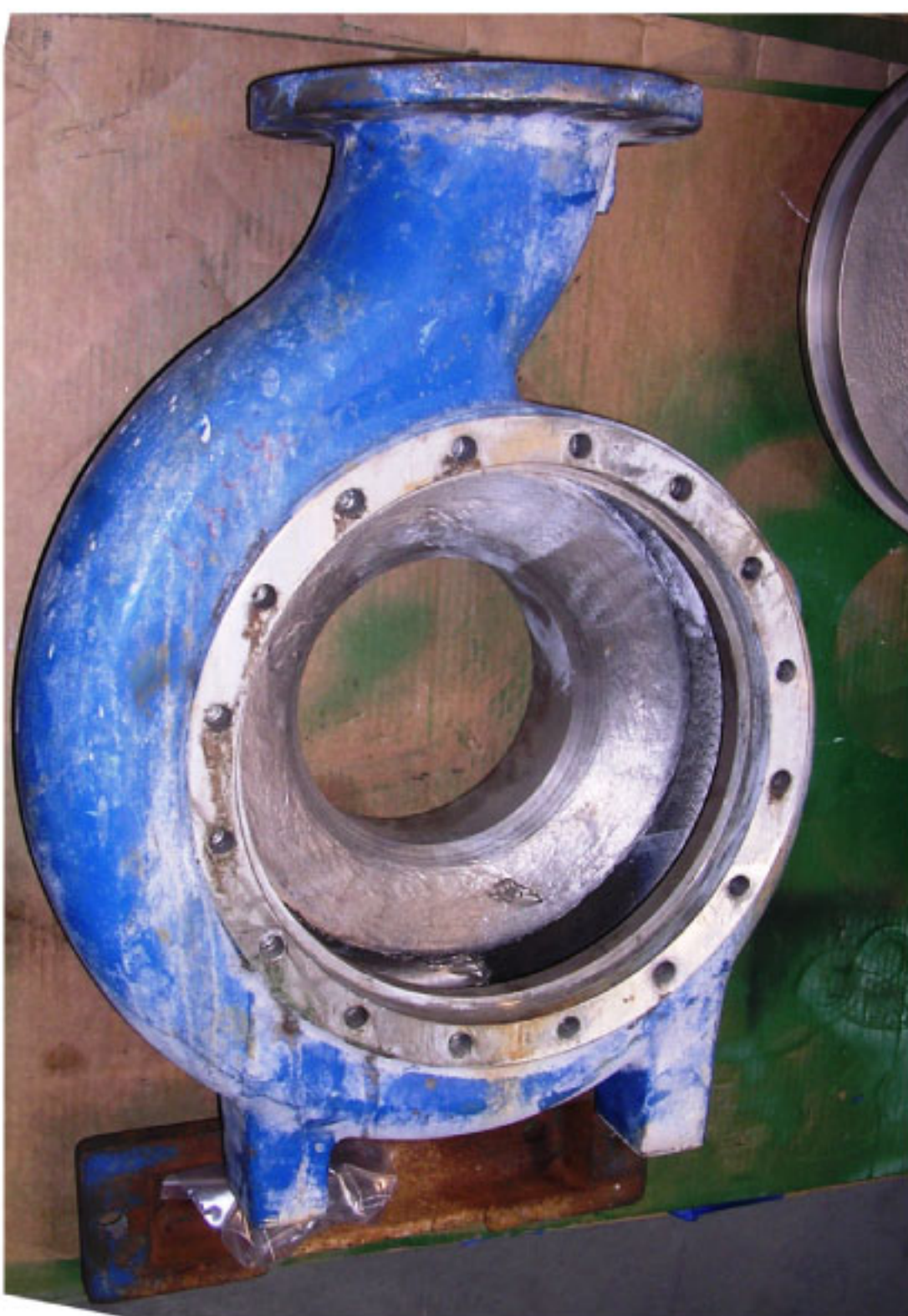
Casing Before Repair
