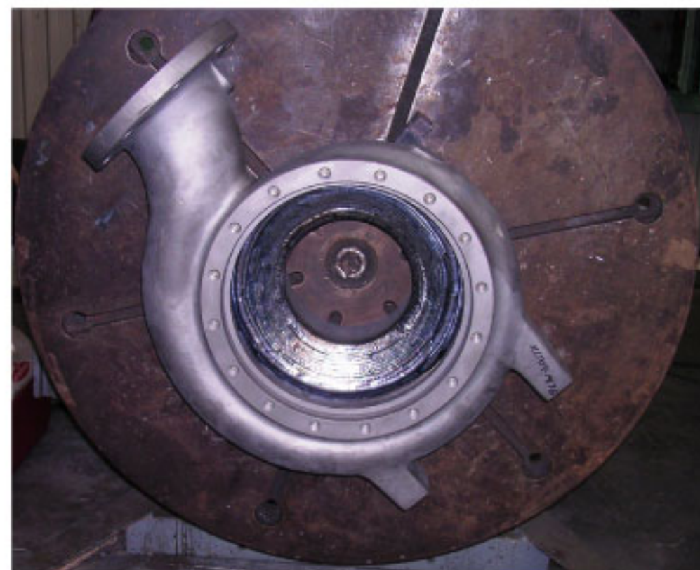
Welded Eroded Areas
